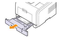
Remove the jammed paper by gently pulling it straight out. Make sure that all of the paper is properly aligned in the tray 1.
